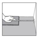
a. Choose the longest and straightest boards and align the planks tongue with the working line, cut the last plank to the proper length leaving a 1/4" from the end wall. Repeat this step for the second row, making sure to stagger the joints. The minimum end stagger is 6 inches.
